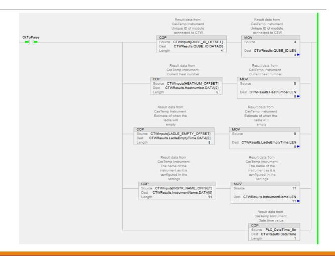
The HEN AOI Encapsulates: Parse the Text Based Results - Error Present
