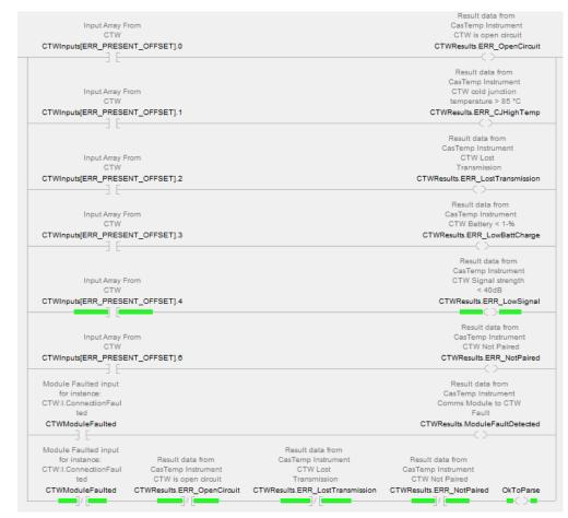
The HEN AOI Encapsulates: Parse the Text Based Results - No errors
