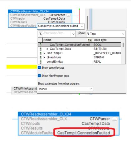
CTWModuleFaulted Parameter for Generic Module Configuration
